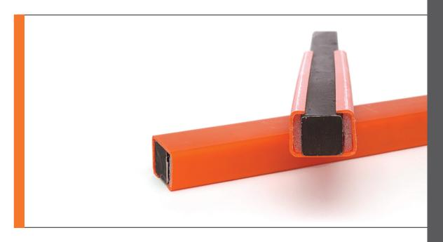
PNA's Square Dowel and Square Dowel Clip™ improve joint stability for reliable construction joints in new and new-to-existing concrete flatwork applications. When paired with the square dowel, the compressible foam inside of the Square Dowel Clip™ allows for joint activation and free horizontal movement of the concrete without restraint. When using this system in new concrete, our Square Dowel Aligners can be used to secure the dowels to wood formwork.
